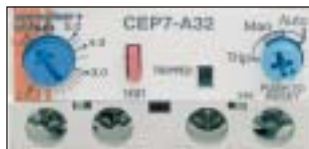
Trip current, manual trip and reset controls are easily accessible
